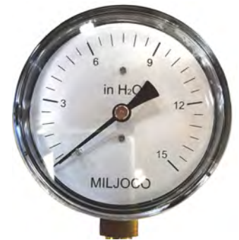
Figure 5 A close up of the Water Column Gauge on a Laguna Gas Kiln
