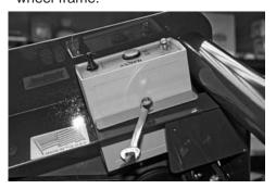
At some point you may need to send your control box or foot pedal in for repair or replacement. Axner has made these components easy to remove, so the heavy frame does not have to ship.
