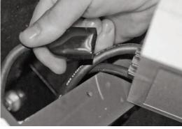
C. Bring the foot pedal up under the wheel. Then carefully pass it out through the hole where the control box sat. Now you can send the box and the pedal.
