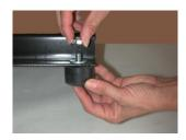
Take your Clay Plunger; and attach it to the back of the Clay Hopper. You must unscrew the nuts before attaching as shown in the picture, then simply slide the Clay Plunger onto the bolts and replace and tighten the nuts you have just removed.
