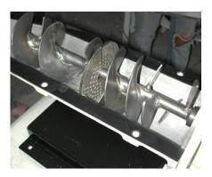
Remove the screen by rotating the two pieces until one comes off from the top.
