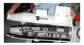
Set in a groove is the shredder screen (shown below)
